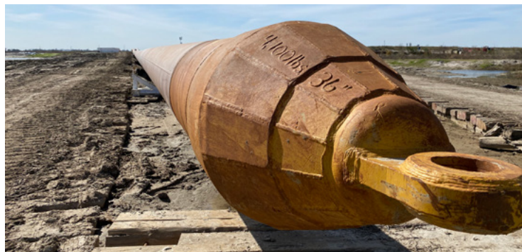
The two-ton reamer that cleared the pipeline path dozens of feet below the Ship Channel.
